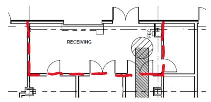
Sometimes, AVB is needed on the interior of the building to seal the building envelope
