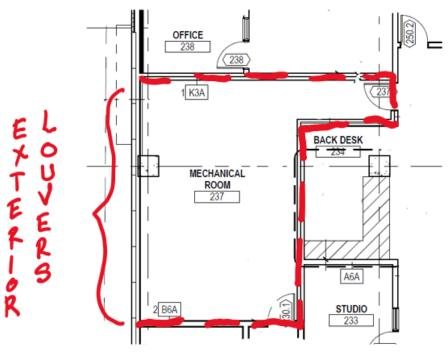
Careful detailing to connect the exterior air barrier with the interior air barrier is needed...
